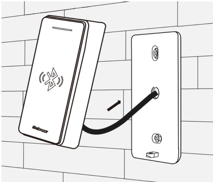
Put the outlet cables through the  $\Phi 10\text{mm}$  hole and connect the needed cables.(Pack the useless cables with the insulating tape.)
