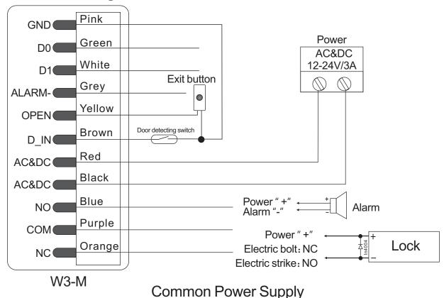
Power DC12V/3A Pink **GND** COM NO +12V GND OPEN Green Wiegand D0 D0 White Wiegand D1 D1 Exit button Grey ALARM-Fail-secure lock Yellow **OPEN** Brown Door detecting switch D IN Alarm "-" Red AC&DC Black AC&DC**■** Blue NO Purple COM( Orange NC
