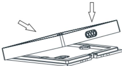
When disassemble the exit button. Press the middle part of the back housing and pull it upward. Pull out all the wires then you can take out the front housing. Please check the below pictures.
